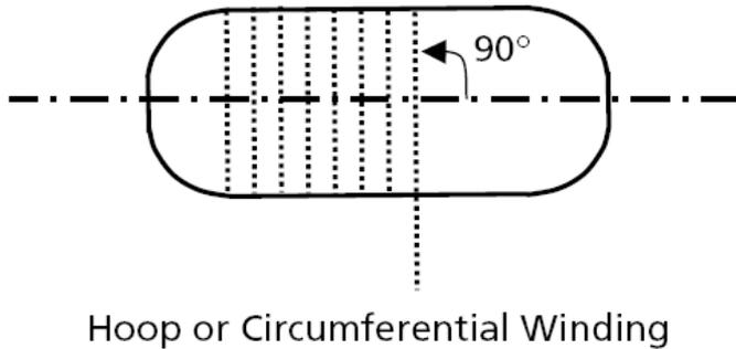
Reinforcement of cylindrical part
