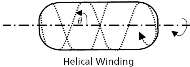
Helical angle chosen to make geodesic winding
