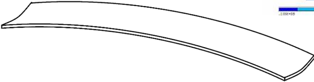
7.4 Curvature in (0/90) unsymmetric laminate due to residual thermal stresses.
